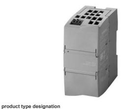
Compact Switch Module CSM 1277 for connecting SIMATIC S7-1200 and up to 3 further nodes to Industrial Ethernet with 10/100 Mbit/s; unmanaged switch, 4 RJ45 ports, ext. 24 V DC power supply LED diagnostics, S7-1200 module incl. electronic Equipment Manual on CD-ROM.
