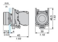
e : clamping thickness: 1 to 6 mm / 0.04 to 0.24 in.
